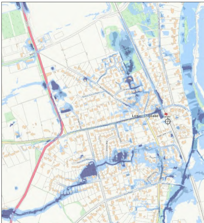
Figure DG6: Plan highlighting the surface water flooding issues in Lower Shiplake (darker blue are areas at high risk of surface water flooding)
