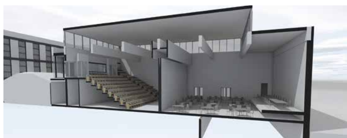
The hall could also be split in two with a lowered acoustic screen for using as two teaching spaces. This could provide a 250 seat lecture theatre, with separate space for further teaching
